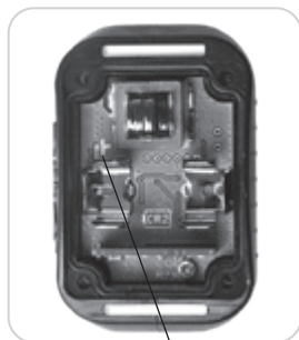
Battery polarity indicator
