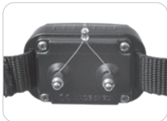
Figure indicating the test lamp attached
